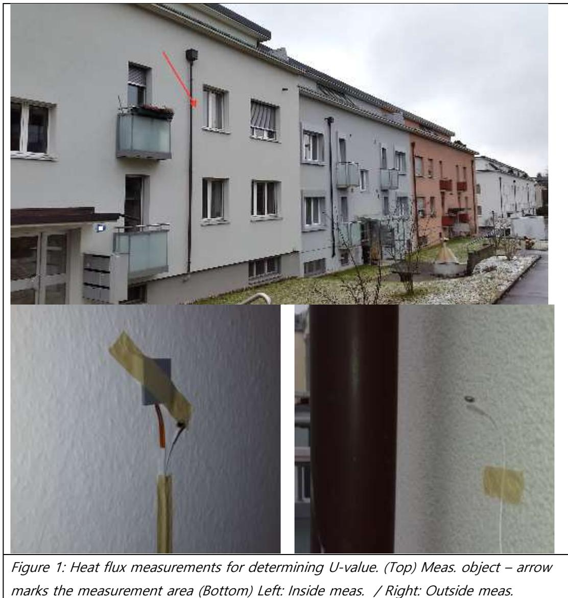
Figure 1: Heat flux measurements for determining U-value. (Top) Meas. object – arrow marks the measurement area (Bottom) Left: Inside meas. / Right: Outside meas.
