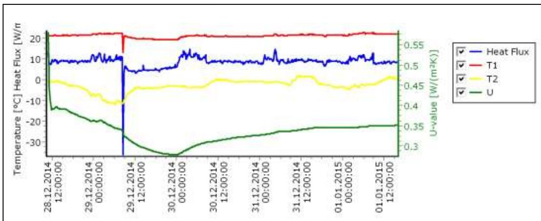
Figure 2: Results at constant conditions according to ISO 9869 (Report obtained from greenTEG Software v0.01.07, 2014)
