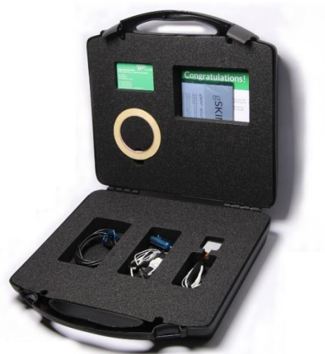
Figure 1: U-Value KIT in transportation box
