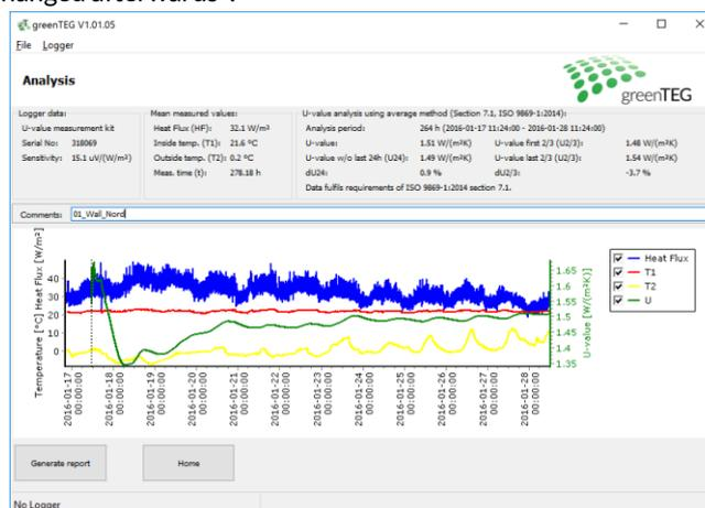
Figure 3: Analysis window showing U-value output and sensor data graphs.
